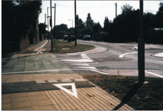
**Photo 3.13.3: Off carriageway cycle facilities at a mini-roundabout**
