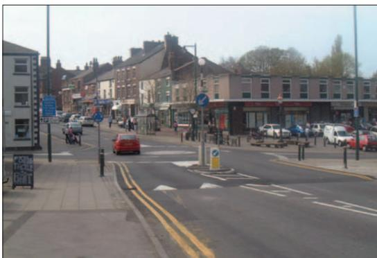
**Photo 3.6.3: Mini-roundabout on raised junction**
