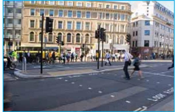
Staggered signalised crossing without guardrail
