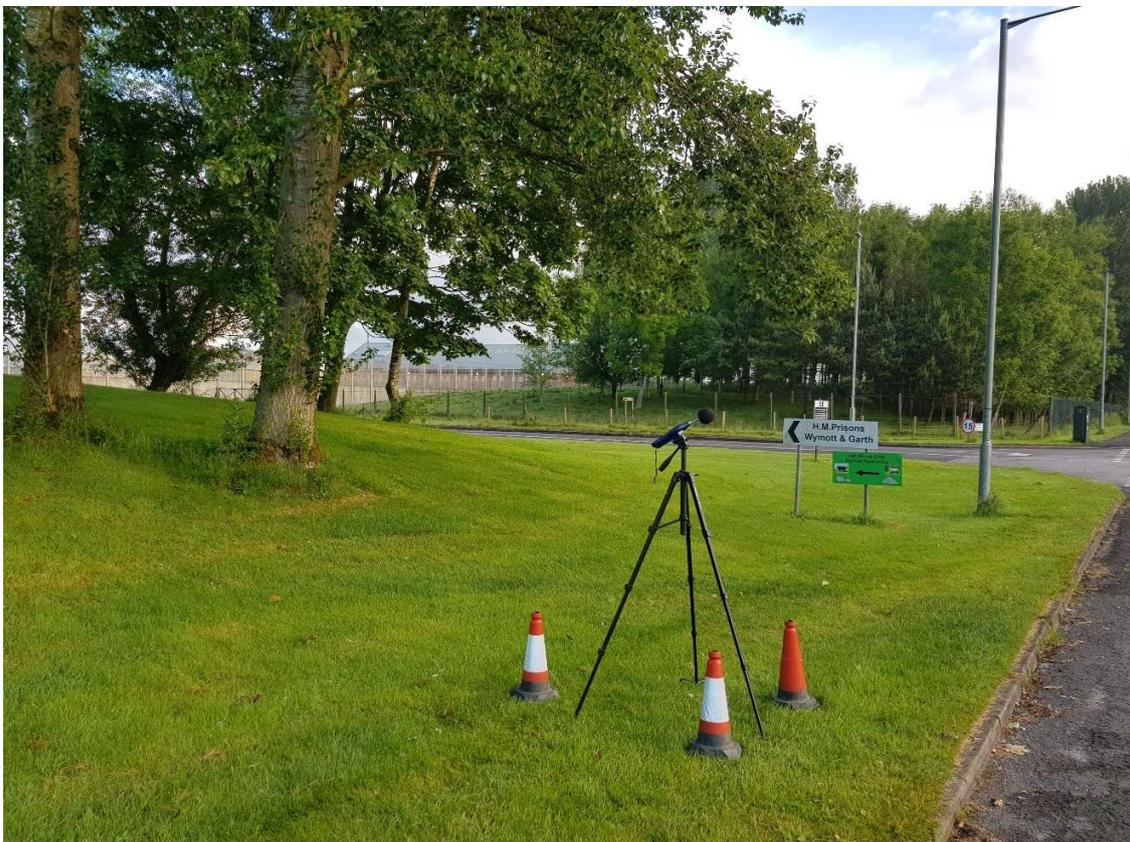
Picture 1: Measurements conducted with a class 1 sound level meter (junction with HM Prison road)
